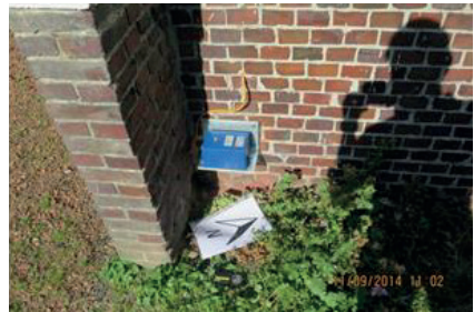
Figure 5. Examples of the 400+ accelerometers installed on a steel bracket and above ground level (taken from Bommer et al, 2018)
