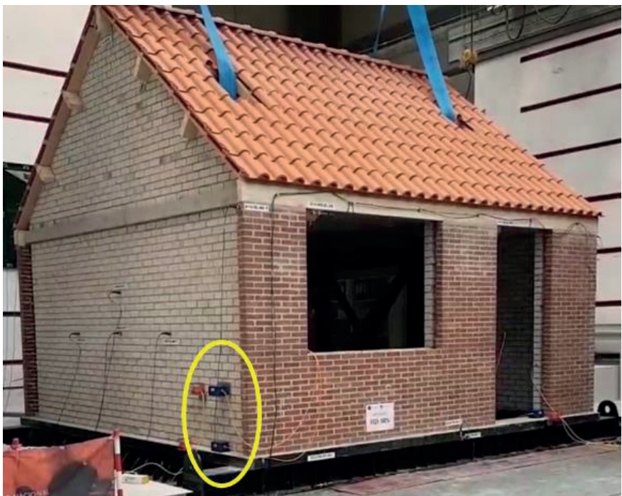
Figure 6. Reproduction of the installation of accelerometers at ground level and at a higher level on a full-scale shake table model at LNEC, Portugal (taken from Bommer et al., 2018)
